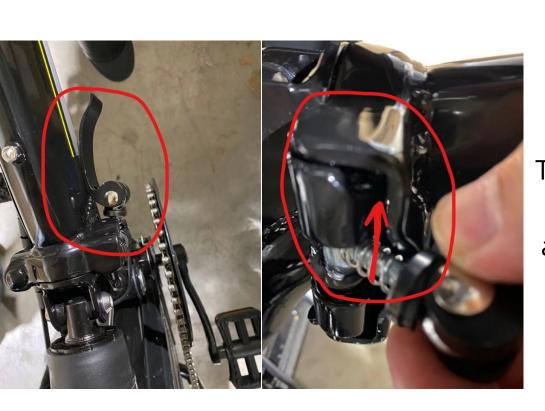
To fold the bike in half, put it into the first picture's position, then lift it up to the arrow direction, then fold the entire bike.
