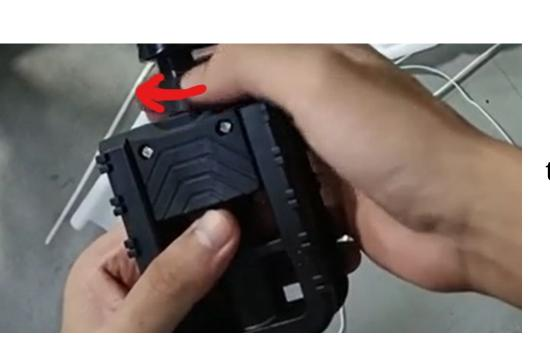
The foot pedals can be installed by just tightening the foot pedal to the direction shown.
