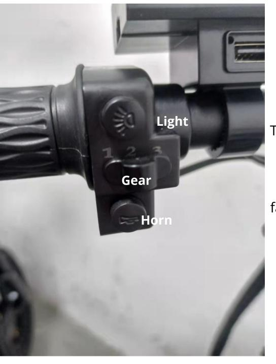
There are two buttons and one switch located on on the left-hand side handle. Two buttons are for the LED light and horn and a switch is for the max speed For the speed switch, there are three different settings, 1 is the ECO & 3 is the fastest. Depending on which one is chosen this will limit the max speed on the bike when using the throttle.
