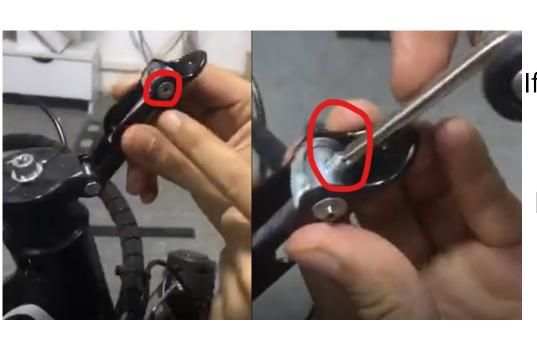
If the front bar is too tight/loose to fold, you can adjust the folding mechanism by loosening the screw as shown in the first picture and adjust the screw in the second picture. After it's been adjusted, you can tighten the screw in the first picture.
